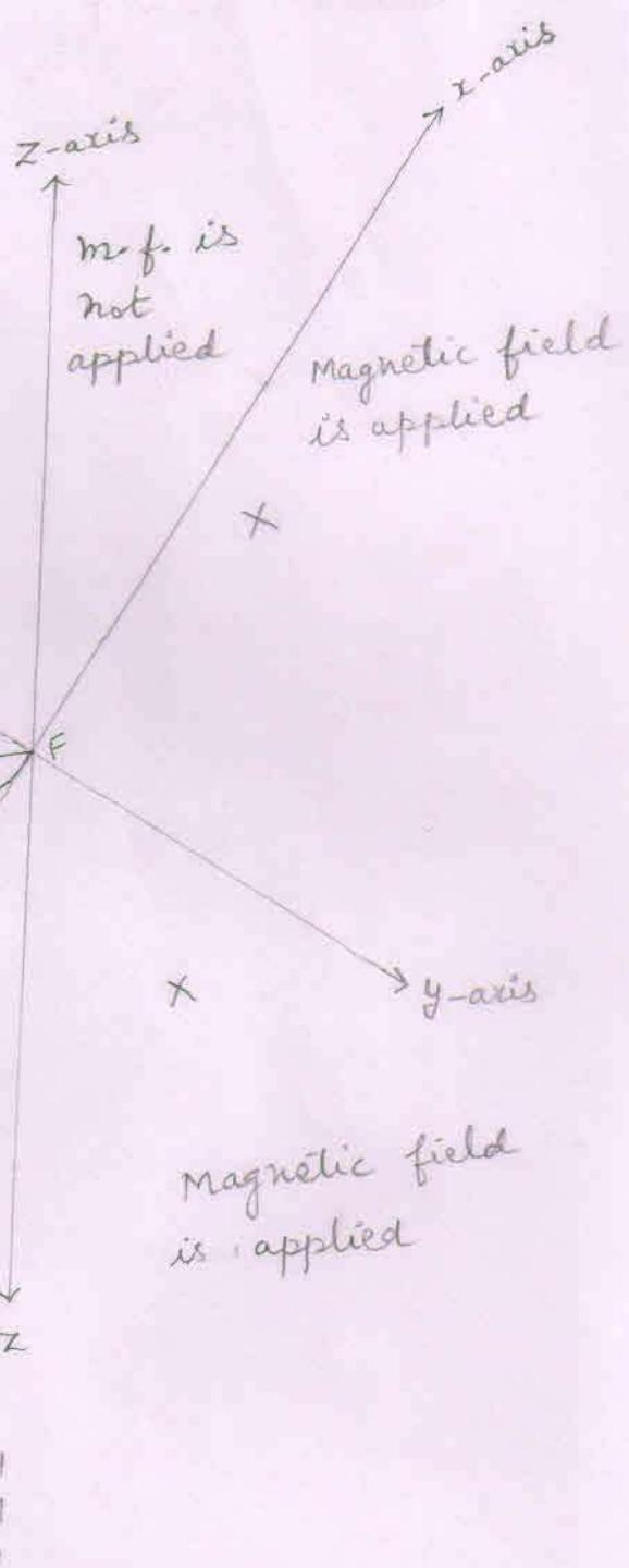
⇒ In trying to follow the confined circular orbit, the proton reaches in a region made-up of negative x-axis and negative y-axis where the magnetic fields are not applied. So, as the proton get rid of the magnetic fields, it starts its linear motion leaving the circular motion.
