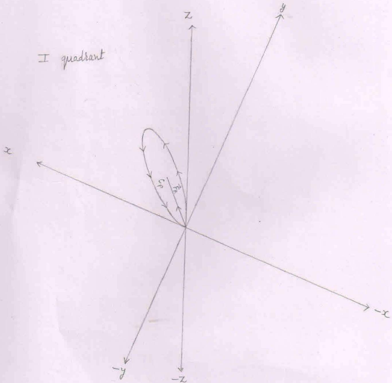
Angles that make the resultant force ( $F_R$ ) [acting on the proton when the proton is at point 'F' ] with positive x, y and z-axes.
